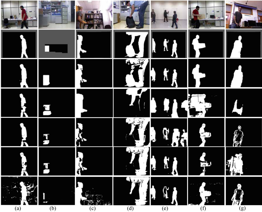
Fig. 3. Visual results of the SRPCA algorithm [1] in comparison with four state-of-the-art subspace learning methods on the SBM-RGBD dataset [25] using intensity features. From left to Right: (a) sequence ‘genSeq1’ from category ‘Illumination Changes’, (b) ‘colorCam1y’ from ‘Color Camouflage’, (c) ‘Despatx_ds’ from ‘Depth Camouflage’, (d) ‘movedBackground2’ from ‘Intermittent Motion’, (e) ‘MultiPeople2’ from ‘Out of Sensor Range’, (f) ‘genSeq2’ from ‘Shadows’, and (g) ‘Bootstrapping_ds’ from ‘Bootstrapping’. From top to bottom: seven input images, ground truth images, the results obtained by SRPCA algorithm, DECOLOR [19], 2PRPCA [14], 3TD [17], and BS-GFL [20].
