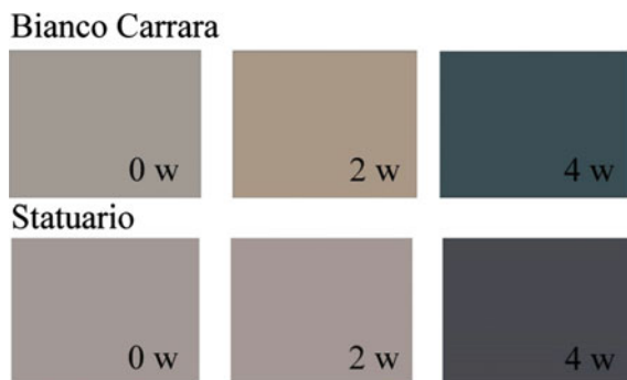
Fig. 19.2 Surface color ( L^*a^*b^* ) at (0w) 0 weeks of exposure to aging, (2w) 2 weeks of exposure, and (4w) 4 weeks of exposure, for both Bianco Carrara and Statuario marbles
