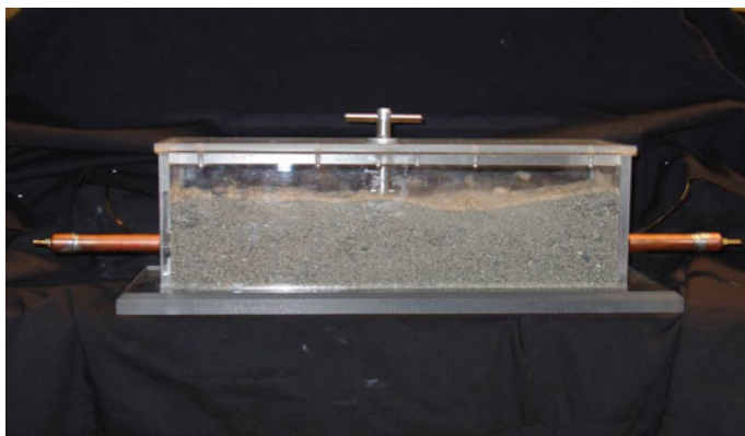
Fig. 14.4 Leak-detection test chamber: copper pipe with leak valve passes through the chamber. Fiber optic cable passes along the side of the copper pipe with 4 cm of evanescent field sensing length near the leak location
