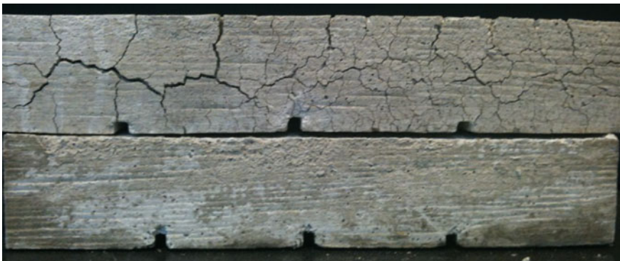
Fig. 16.4 Images of bar samples after and before degradation, showing location of notches where the
