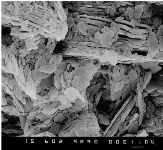
Fig. 5.2 Kaolin plates and stacks (Murray 2000)
