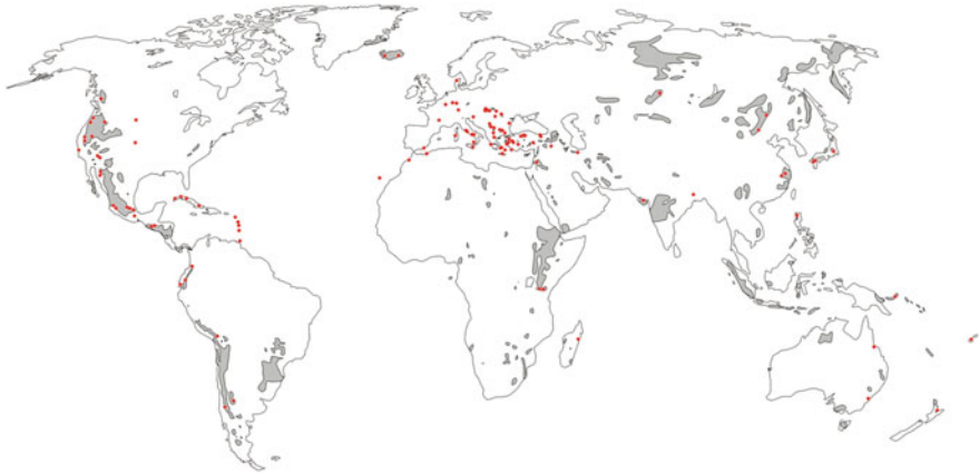
Fig. 6.4 Global distribution of volcanic rocks (grey areas) and deposits of reported natural pozzolans (black dots) (Snellings et al. 2012)
