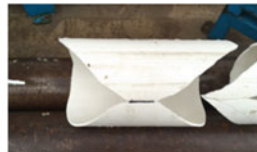
Photo 8. PVC pipe failure
