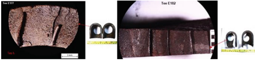
Fig. 4 Fracture surfaces are observed in both parts, the steps and the null plastic deformation associated to the fracture are observed
