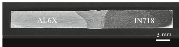
Fig. 3 Profile of dissimilar weldment IN718-AL6XN
