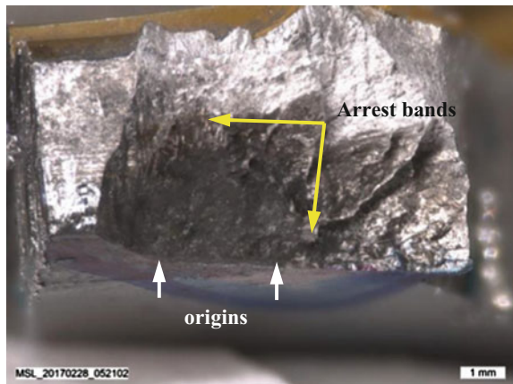
Fig. 4 Fracture surface of crack on bolt hole #24
