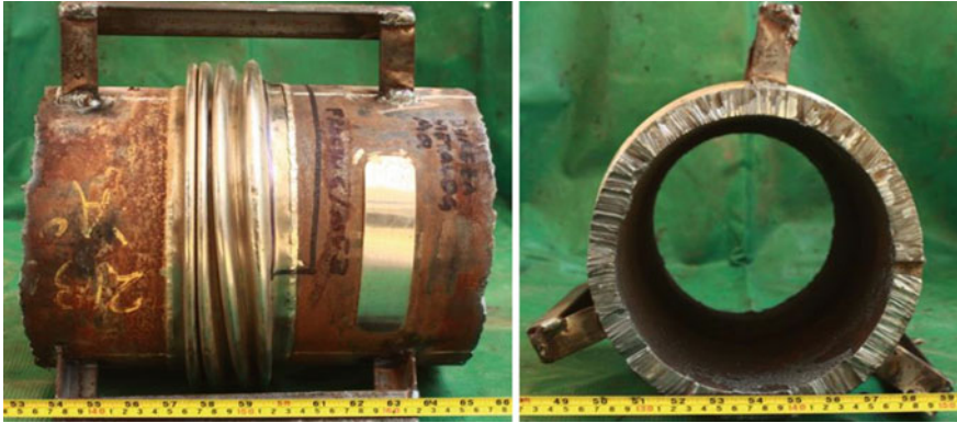
Fig. 2 Expansion joint in the condition as it was received for study in the Laboratories of the DIMM-IPN
