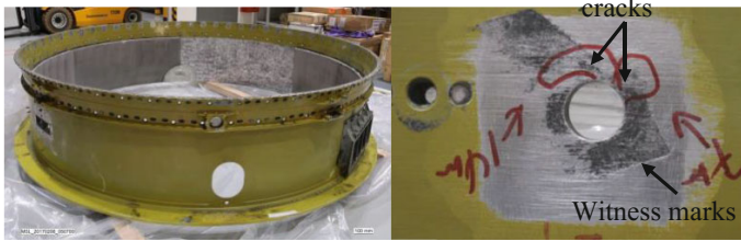
Fig. 1 Overview (left) and close-up (right) showing contact witness mark and fretting around the vane bolt holes. The typical parabolic shape of the cracks was also shown
