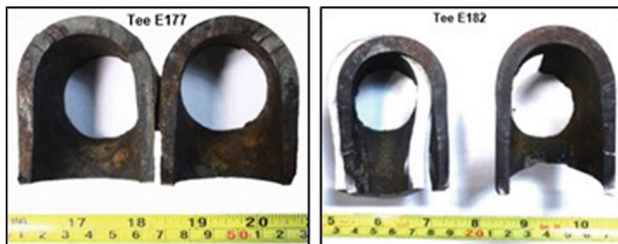
Fig. 3 Fracture surface observed on Tee E177 and Tee E182 respectively. Note the steps and the null plastic deformation in both samples
