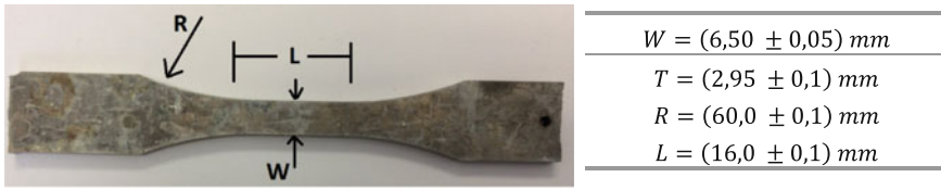
Fig. 2 Uniaxial tensile fatigue specimen size
