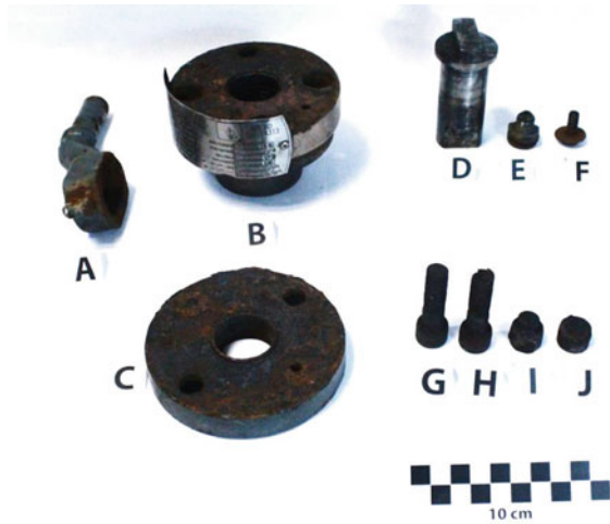
Fig. 1 Disassembling the bonnet, the elements named G, H, I and J, correspond to the failed screws
