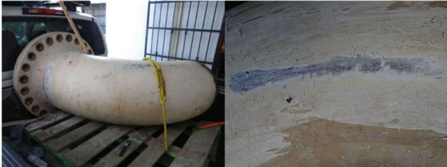
Fig. 1 Long radio elbow removed from Spool due to cracking
