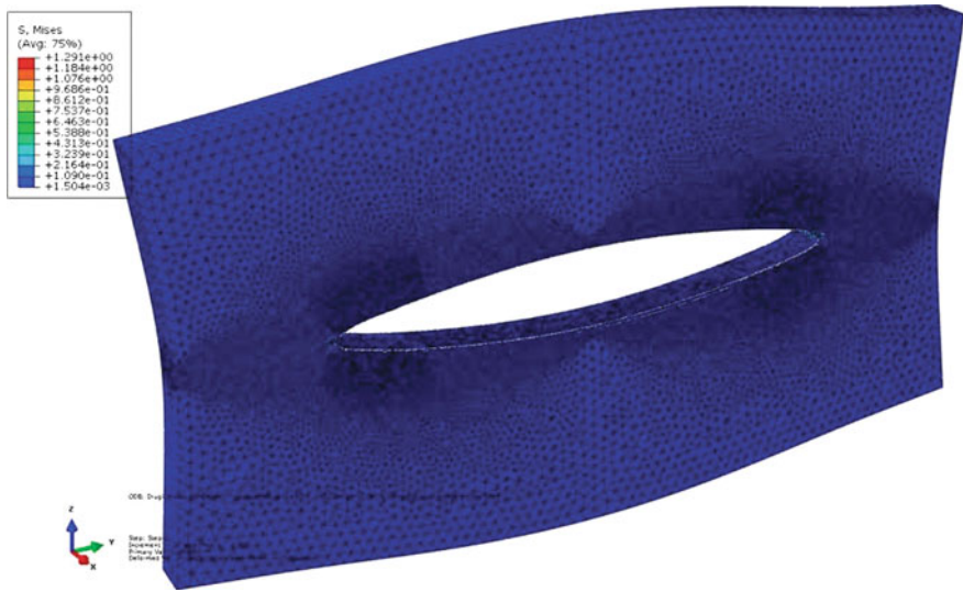
Fig. 10 Stress state (von Mises) of a plate after 18 steps of crack propagation (tetrahedral elements)
