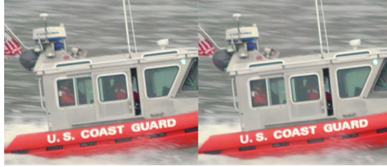
Fig. 2. Illustrative example of the performances of the new JND-guided pre-filters (Coast guard sequence, QP28): original and BilAWA pre-filtered version with a bit rate saving of about 30%.
