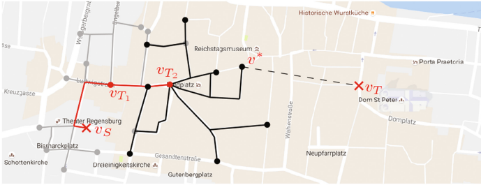
Fig. 2. The subgraph G_3^* is depicted in black, whereas the subgraphs G_1^* and G_2^* are grey. The already calculated routes R_1 and R_2 are red. The vertex v^* has the lowest straight-line distance |v^* - v_T| to the overall target v_T and will be used as the next step v_{T_3} . (Color figure online)
