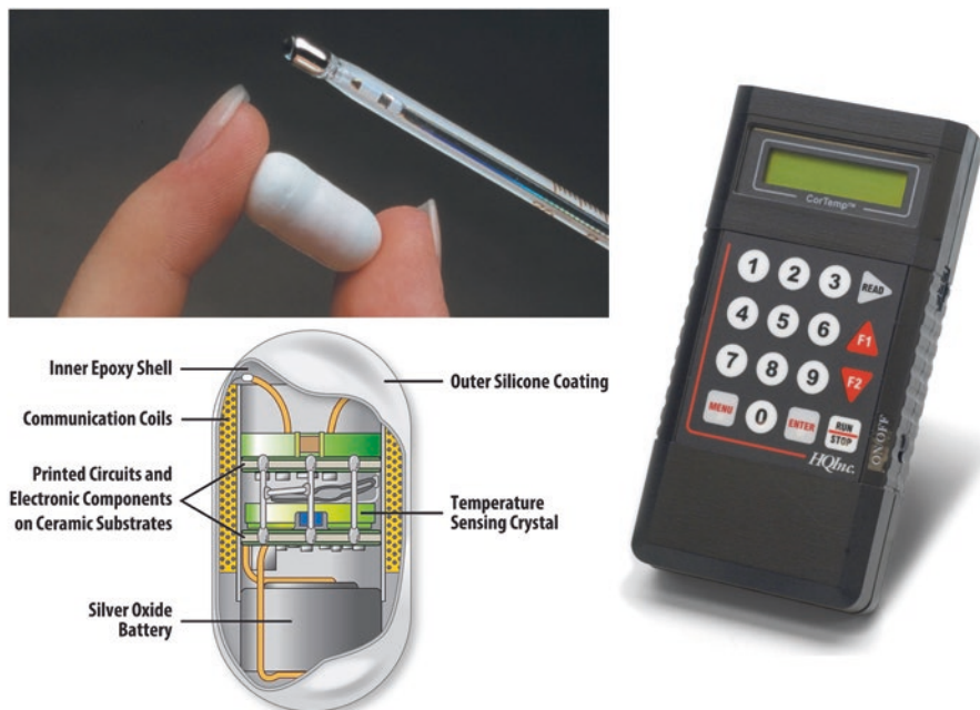
Fig. 10.1 HQInc ingestible thermometer pill and data logger [50]. Copyright © HQ, Inc. Reprinted by permission
