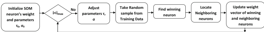
Fig. 1. Traditional approach for SOM training. Here \eta_0 : initial learning rate, \sigma_0 : initial neighborhood size, \eta and \sigma are continuously decreasing functions at each iteration, i_{max} is the maximum number of iterations for SOM training
