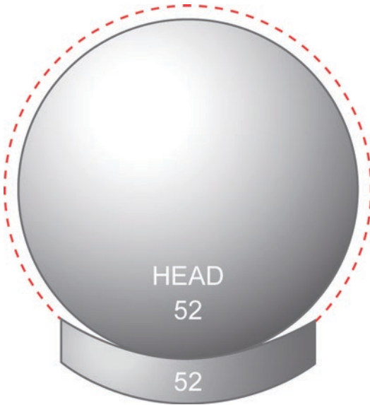
Fig. 13.1 Typical mismatch between the radius of curvatures of the humerus and glenoid component
