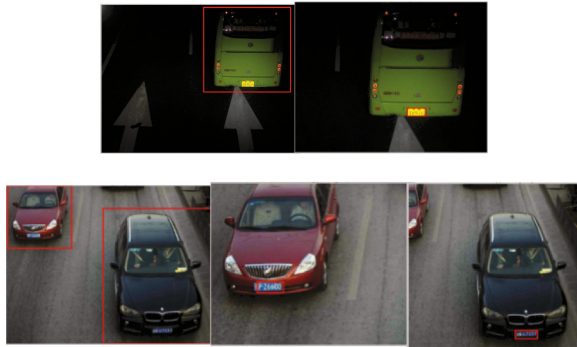
Fig. 4. Some of successful results. Red bounding boxes labeled in the first picture in each line are the vehicle proposal. The boxes in remaining pictures in each group are the detected locations of license plates in the corresponding vehicle proposals. Better viewed by zooming. (Color figure online)
