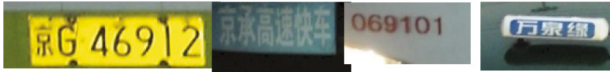
Fig. 6. Some of the proposals extracted from stage 2 of the proposed CNN. Only the first image is recognized as the license plate and the other are regarded as the background.
