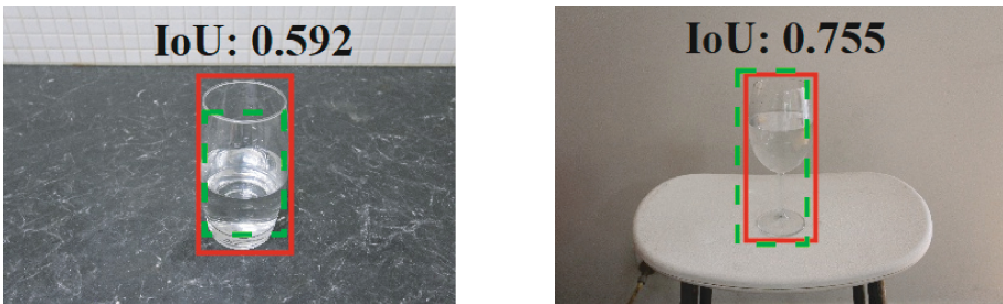
Fig. 1. Example IoU values of a detection where solid line box is the target bounding box and dashed line box is the network output.
