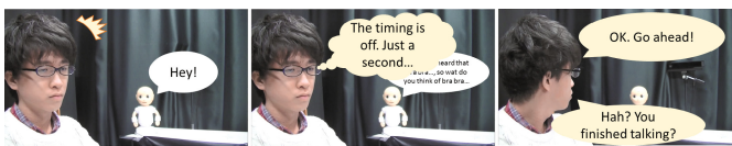
Fig. 1. The failure case of starting a conversation by a recognition failure. In the first scene, the robot says “Hey” to attract the user’s attention. Then, the robot waits for the user and is ready to listen, but the robot misrecognized the user’s state as being ready to listen and started to speak on a main topic. As a result, the user missed what the robot said.
