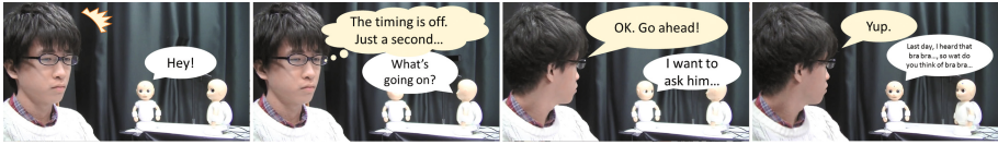
Fig. 2. The proposed behavior pattern between two robots before starting a conversation.
