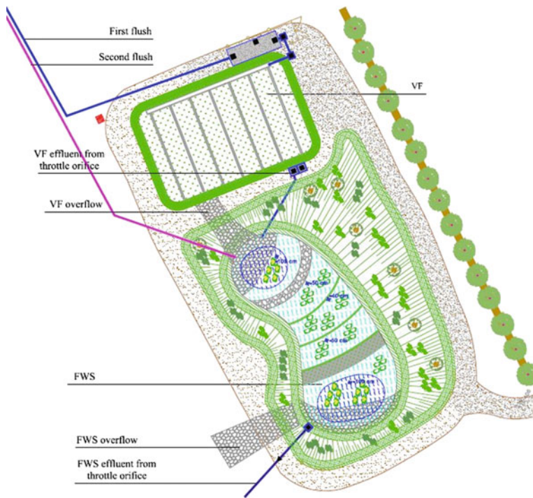
Fig. 7.8 CSO-CW system designed for Capiago Intimiano (Italy), with inflows entering from the top and outflows from the bottom left of the diagram
