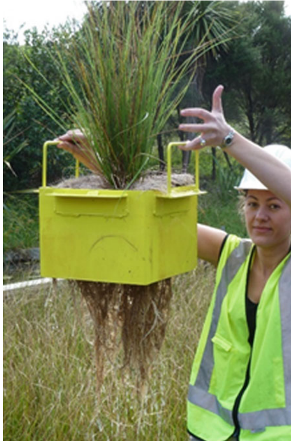
Fig. 2.7 Extracted section of a Floating Treatment Wetland treating road runoff showing root mass extending beneath floating mat (Karine Borne, Auckland, New Zealand) (Photo C. C. Tanner)
