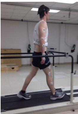
Fig. 2. Experimental setup: data collection for user intent recognition for able-bodied subjects
