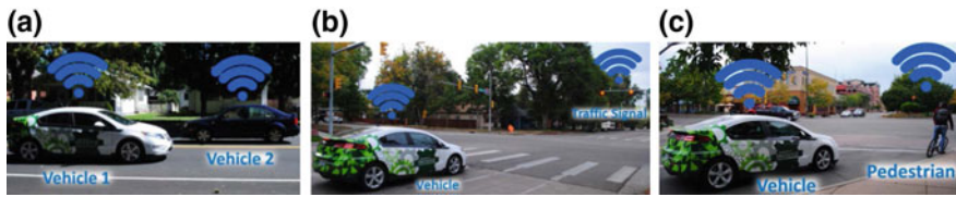
Fig. 3 Conceptual examples of near-future CAV technologies: a V2V, b V2I, and c V2X
