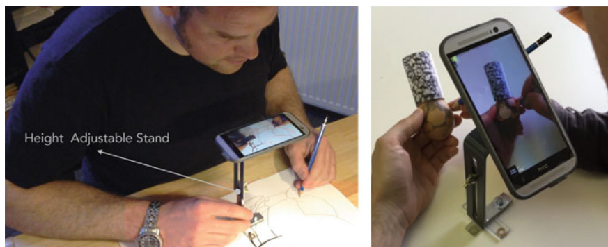
Fig. 18.6 The mobile device renders a virtual template image together with a live video stream of the drawing surface. Left: paper. Right: Easter egg
