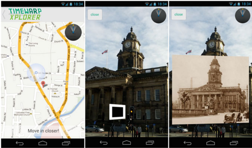
Fig. 18.4 TARX application: map, AR and warp view. TARX has an automatic interface switching implemented, to switch the AR view to a traditional map view based on the orientation of the device to save battery life
