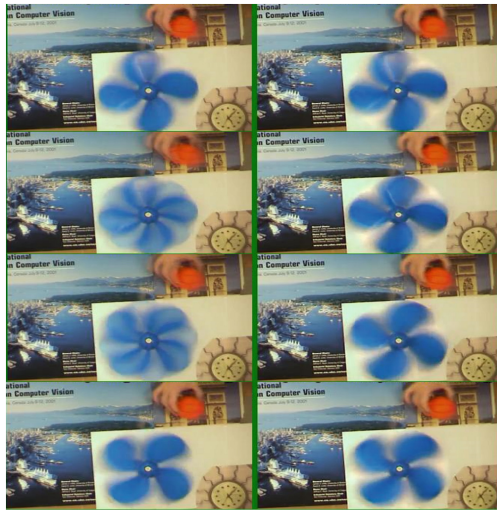
Fig. 4. Temporal SR comparison (3×) between Bayesian approach (left) and our approach (right) [upper and lower one are key frames and mid frames are predicted one]
