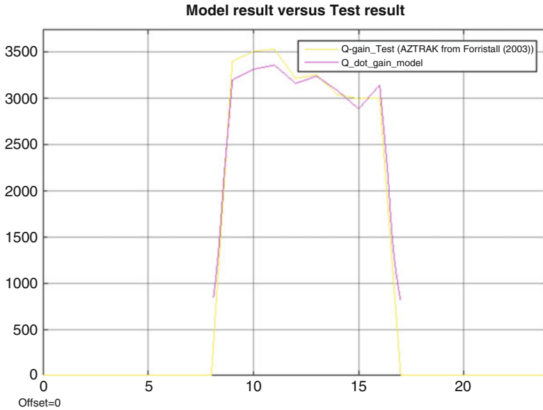
Fig. 28.14 Heat gain (in Watt on vertical axis) of the test model compared to heat gain of the present model over a day (in hours on horizontal axis)
