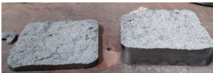
Fig. 8.4 PVA glue as a binder resulted in a split sample upon ejection
