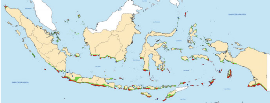
Fig. 21.1 Indonesia wind resource map. Red areas, wind speed average >6 m/s; Green areas, wind speed average 4–6 m/s (P3TKEBTKE 2014)
