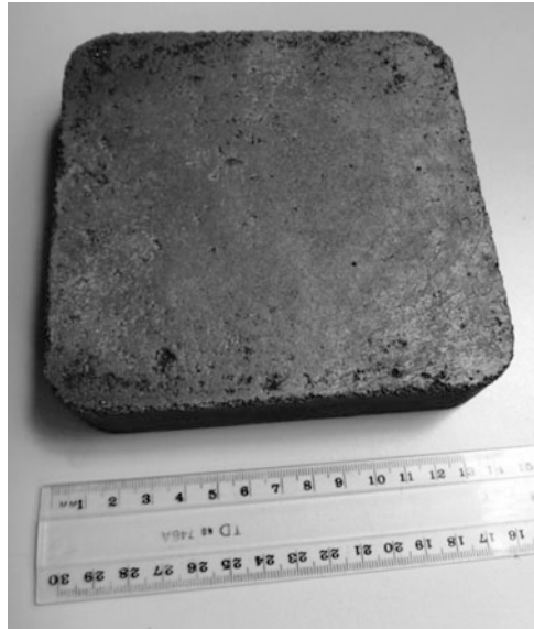
Fig. 48.3 Exterior and interior of large Al-Sn MGA samples showing well dispersed Sn particles in an Al matrix. Dark regions show Sn particles lost during cutting for examination
