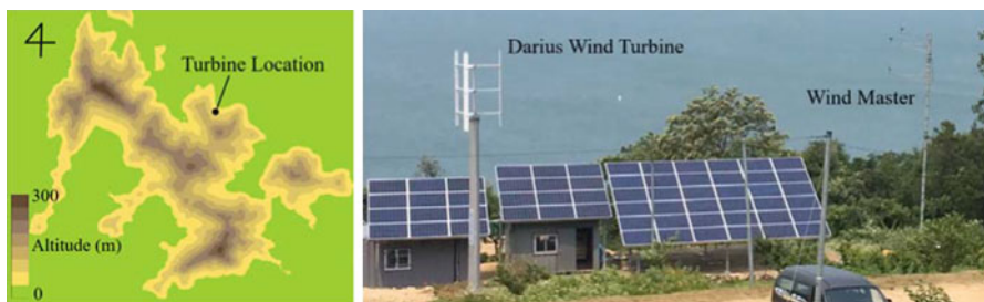
Fig. 18.2 Location of wind turbine with geographical altitude (left) and overall view of system (right)
