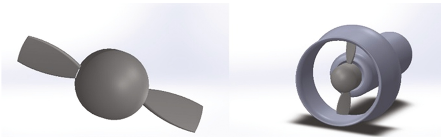
Fig. 4. 3D model of the LBV150 ROV thruster
