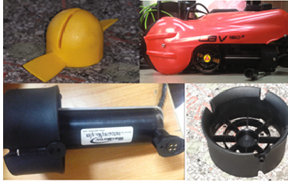
Fig. 1. The SeaBotix LBV150 ROV and its thruster
