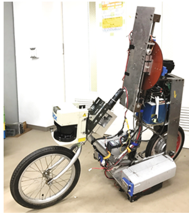
Fig. 1. Unmanned bicycle robot with variable configured balancer.
