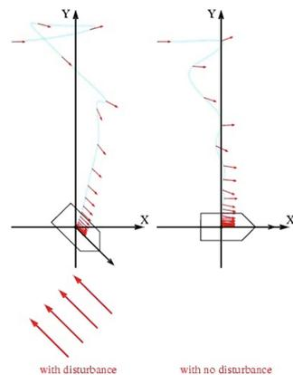
Fig. 7. Surface vessel with tidal stream
