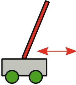
Fig. 8. Conventional inverted pendulum
