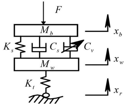
Fig. 11. Semi-active suspension
