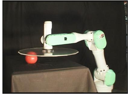
Fig. 4. Dexterous manipulation (ball/plate position)
