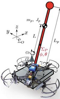
Fig. 10. Inverted pendulum on the drone
