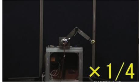
Fig. 13. Under-actuated throwing machine
