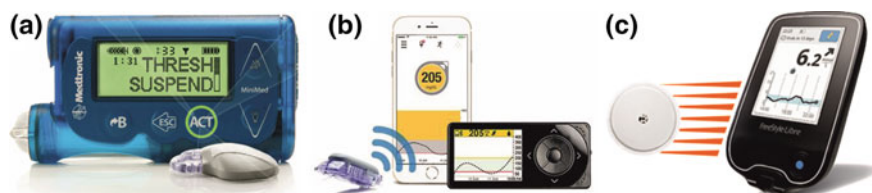
Fig. 2.14 a Medtronic MiniMed 530G pump [208] and Enlite sensor (Given Imaging), b Dexcom S5 CGM [209] (Given Imaging), and c the Abbott Freestyle Libre [210] (Given Imaging). FreeStyle and related brand marks are the trademarks of Abbott Diabetes Care in various jurisdictions
