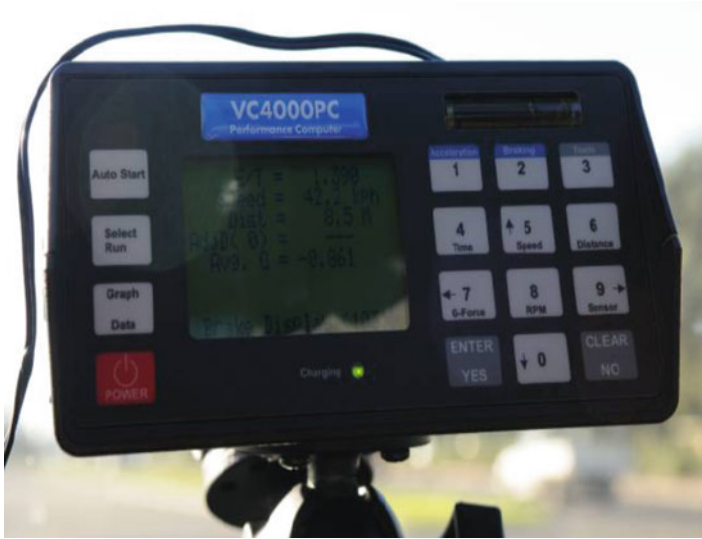
Fig. 8.6 Vericom VC4000PC performance brake test computer with results displayed
