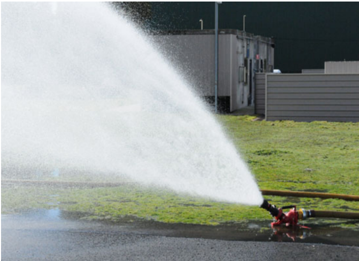
Fig. 8.17 Fire hose pumping water to simulate heavy rainfall conditions
