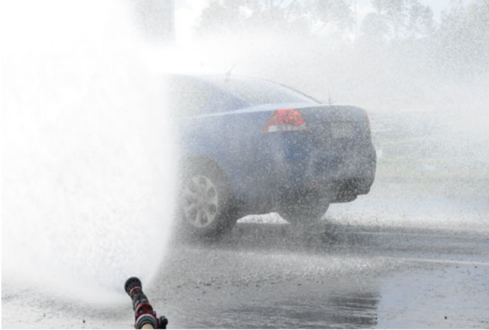
Fig. 8.18 Simulated rainfall direction and vehicle during braking
