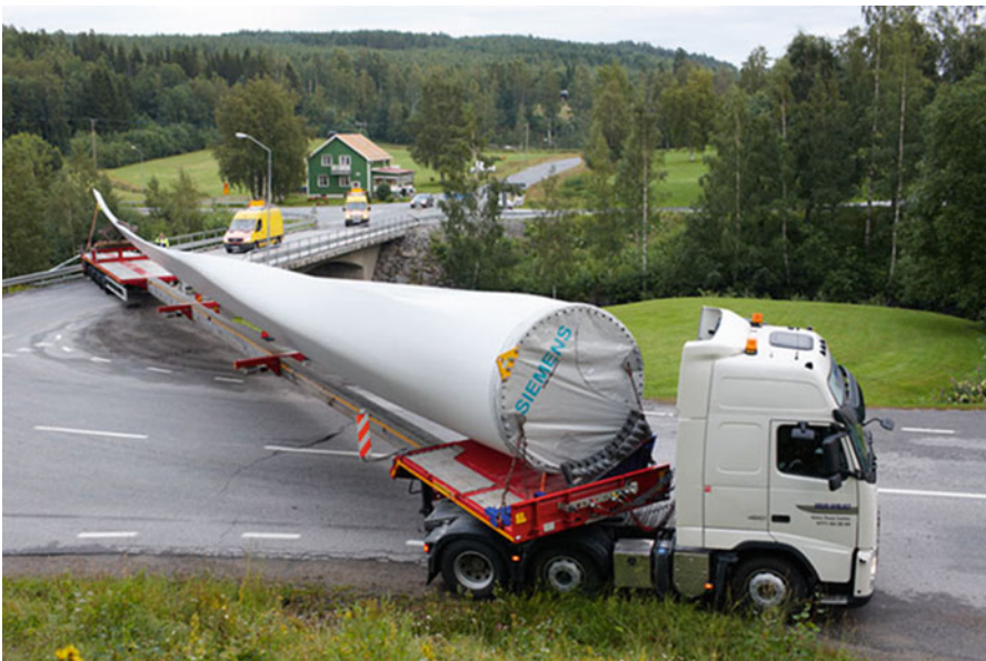
Fig. 1.4 Wind turbine blade in transportation (Statkraft 2012)
