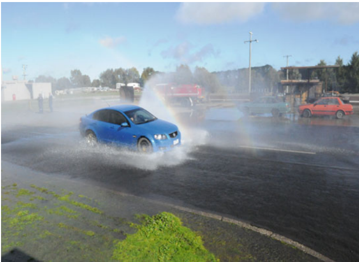
Fig. 8.19 Vehicle during braking throughout simulated rainfall testing
