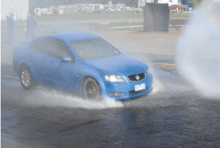
Fig. 8.20 Closer view of vehicle during braking in simulated rainfall testing
