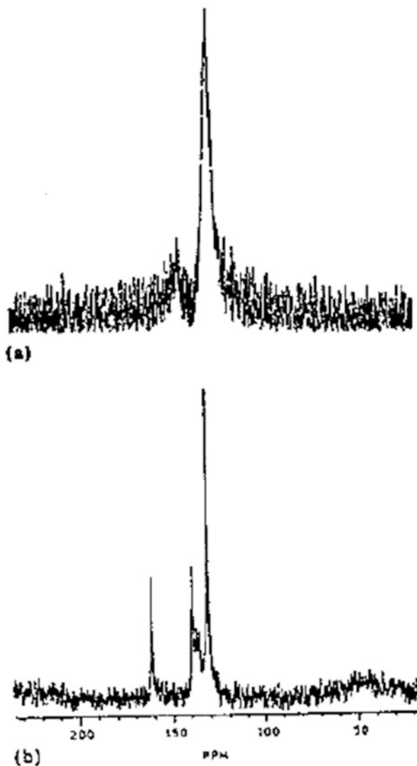
Fig. 33.35 ^{13}\text{C} n.m.r. spectra of the emeraldine salt (a) before and (b) after oxidation in sulfuric acid (After Ref. [1192], reproduced with permission)
