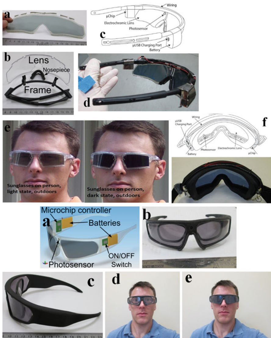
Fig. 38.10 Elements of practical electrochromic sunglasses and goggles using CP-based electrochromics (After Chandrasekhar et al. [1845])
