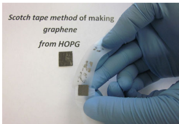
Fig. 16.2 Illustration of the “Scotch® tape” or mechanical exfoliation method of fabricating sheets of single-layer graphene from highly ordered pyrolytic graphite (HOPG) (After Ref. [481], reproduced with permission)
