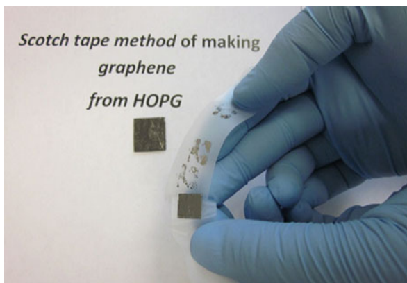
Fig. 18.1 Illustration of the “Scotch® tape” or mechanical exfoliation method of fabricating sheets of single-layer graphene from highly ordered pyrolytic graphite (HOPG) (After Ref. [480], reproduced with permission)
