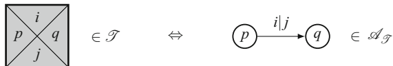
Fig. 10.5 The transducer \mathcal{A}_{\mathcal{T}} associated with a Wang tileset \mathcal{T} according to Culik-Kari.
