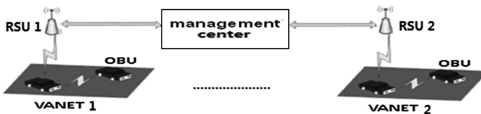
Fig. 1. The basic structure of ITS
