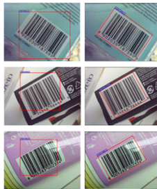
Fig. 6. Detection without angle correction
