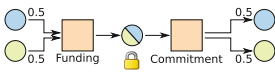
Fig. 1. Construction of a micropayment channel. The boxes are transactions or a number of transactions and the circles are outputs. The colors in the circles describe whose signatures are needed to spend those outputs. To spend an output belonging to multiple parties, all of those parties must sign. The lock indicates unspent transaction outputs on the blockchain while the channel is open. (Color figure online)
