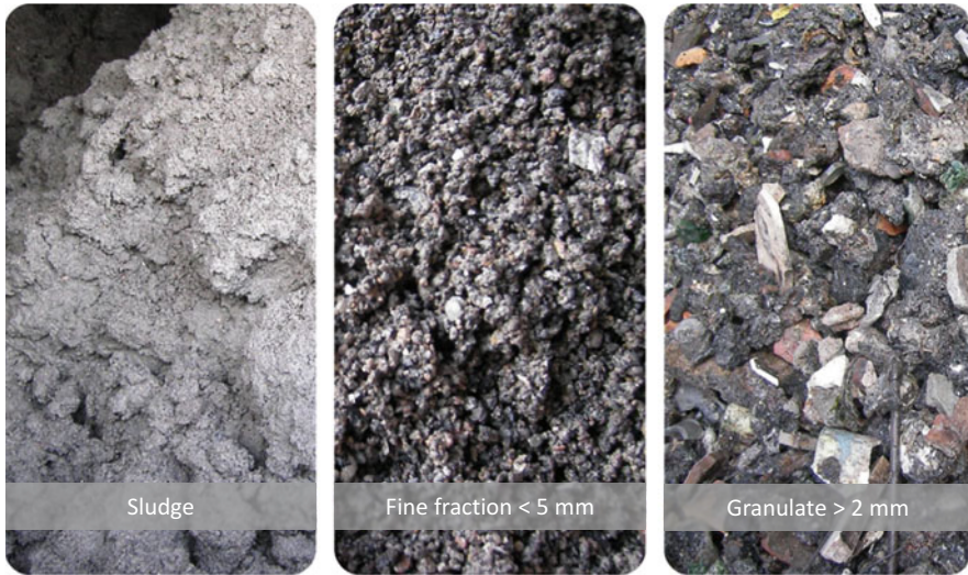
Fig. 9 Granulate product from SYNCOM-Plus process ( right ) and sludge, as well as fine fraction for recycling in the incineration process (Photos Peter Quicker)
