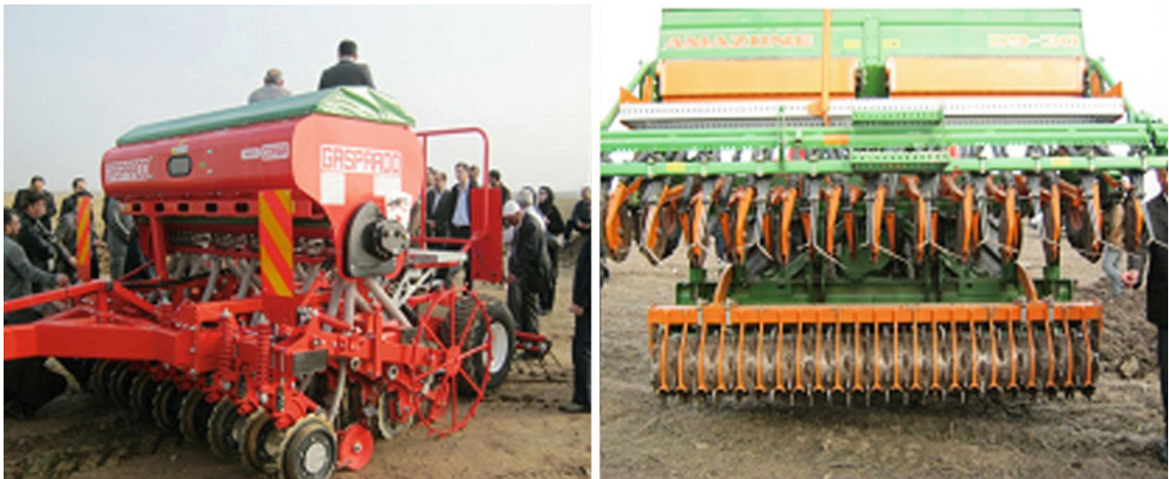
Fig. 13.15 Examples of the imported direct seeders used in direct seeding practices in Iran (courtesy Sayre 2014)
