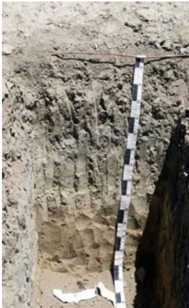
Fig. 7.19 A typical profile of a Torrifluvent developed on the lower terraces of Zayandeh Rud in Isfahan
