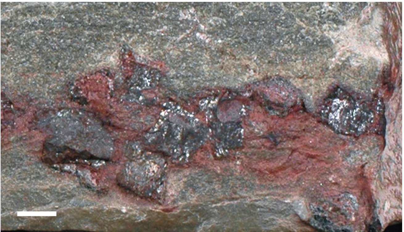
Fig. 23.13 Klein Aub Mine. Angular chalcocite cubes (dark silver) with hematite halos (maroon-red) pseudomorph after pyrite cubes in mineralised meta-arenite (underground 450 m level, stope 600 W, scale is 5 mm). Note that the soft chalcocite has not been deformed and must thus post-date peak deformation. Photograph by Gregor Borg
