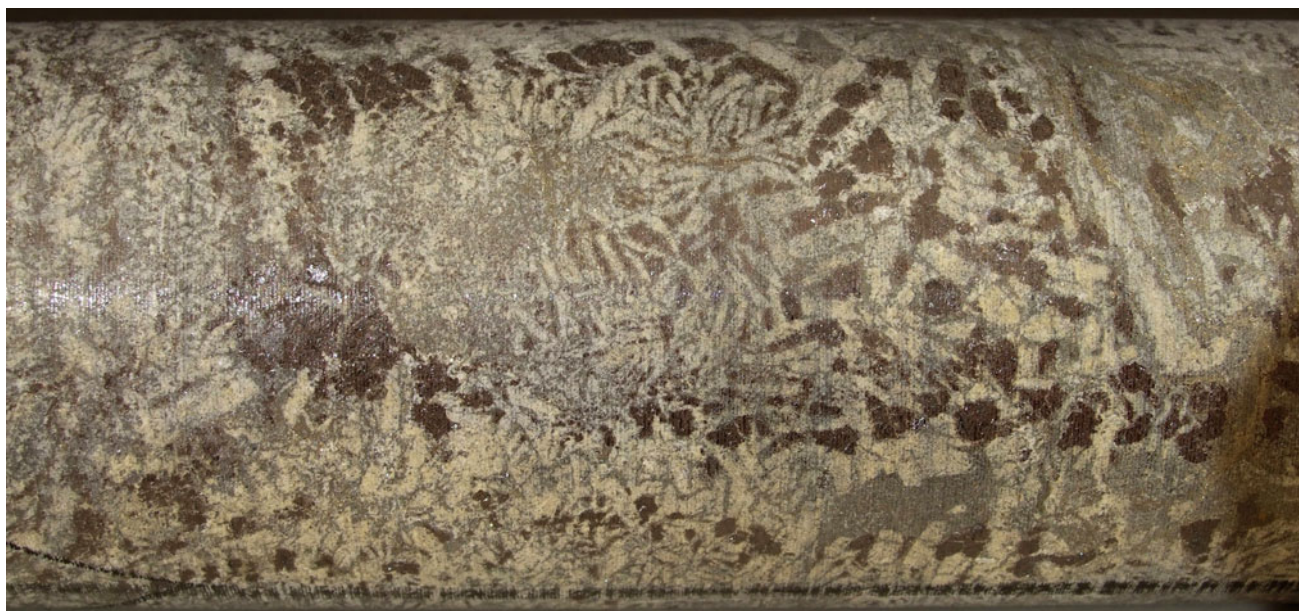
Fig. 23.34 Gergarub drill core with hypogene sphaerite (brown) intergrown with blade-shaped barite (white). Borehole SPDD 48 at 259.70 m depth, core diameter NQ (47.6 mm). Photograph by Gregor Borg
