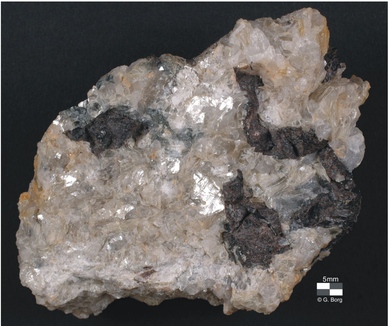
Fig. 23.44 Coarse-crystalline anhedral cassiterite (brownish-black) in quartz-muscovite pegmatite from the Uis tin-pegmatite district, Namibia. Photograph by Gregor Borg
