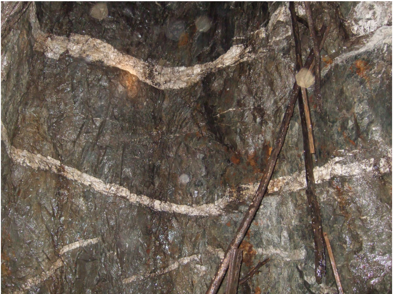
Fig. 23.47 Subhorizontal cassiterite-bearing quartz veins underground at the Vredehoek Mine, Cape Town, South Africa. Width of field of view 1.6 m. Photograph by Gregor Borg
