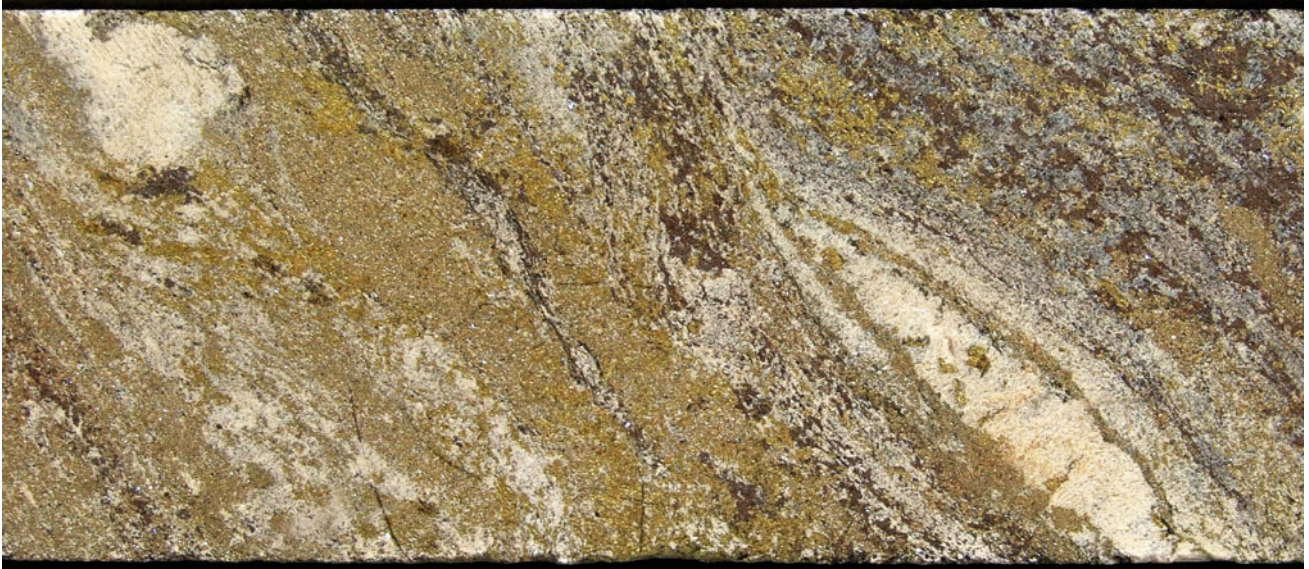
Fig. 23.32 Drill core from the sulphide ore at the Gergarub prospect, Borehole SPDD 31 at approximately 462 m depth, core diameter NQ (47.6 mm). Photograph by Gregor Borg showing rich disseminated to semimassive pyrite-chalcopyrite-sphalerite ore in sheared and metamorphosed hyaloclastic rhyolite.
