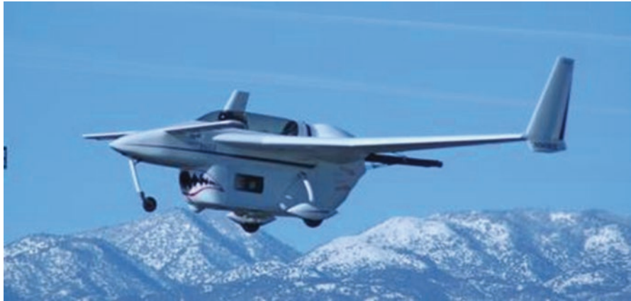
Fig. 6.1 First pulsed detonation powered aircraft, Rutan Long-EZ on Jan 31, 2008 (Heiser and Pratt 2002)
