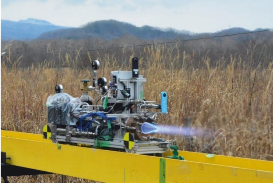
Fig. 4.15 The RDE sled test was successfully performed
