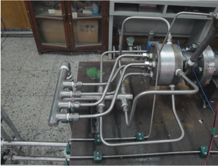
Fig. 7.3 Combustor with pre-detonator
