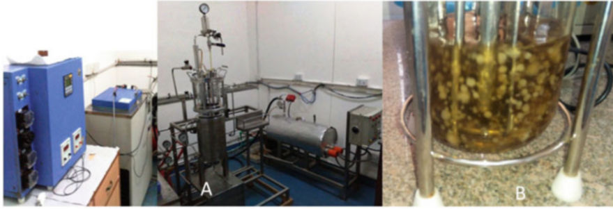
Fig. 19.3 (a) Typical view of a fermenter; (b) P. indica culture in fermenter
