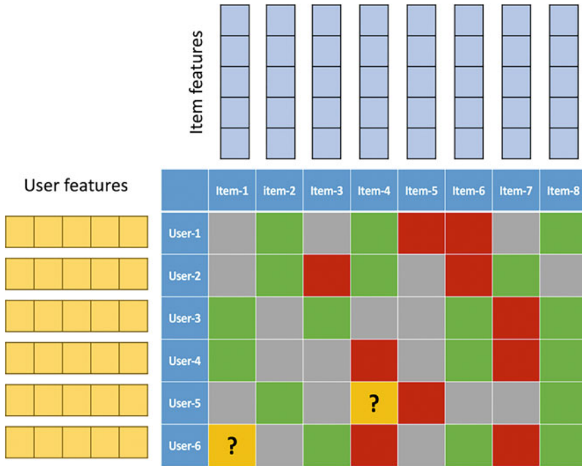
Fig. 16.21 In profile-based recommendation engines, we do not just know the past engagement between users and items, but we also know or infer additional user and item features that can be used to determine which type of users like which type of items
