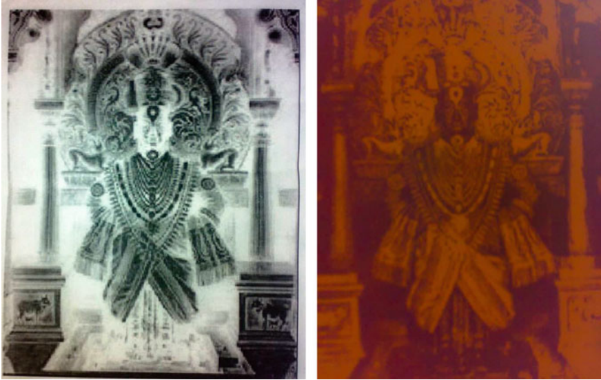
Fig. 23 Grey phototool and 3D pattern developed by the grey PCM
