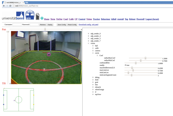
Fig. 8. A screenshot of the web application used to help calibrate the robot.
