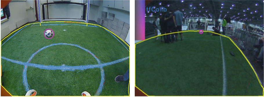
Fig. 5. Left: a captured image with ball (pink circle), field line (light blue lines), field boundary (yellow lines), and goal post (dark blue lines) detections. Right: distant ball detection on RoboCup 2016 field. (Color figure online)
