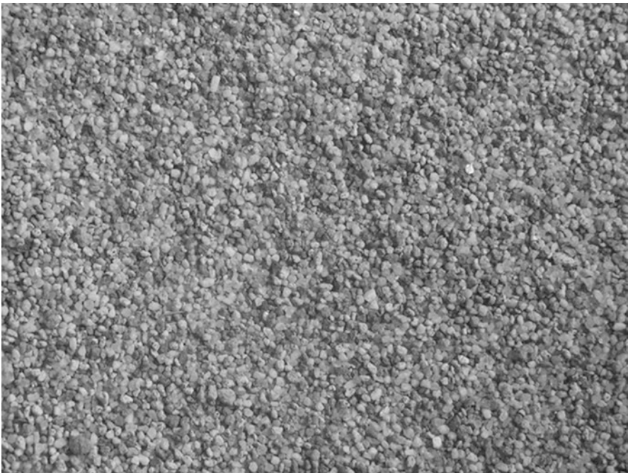
Fig. 10.1 Lahar (10 \times ) consists of sandy aggregates prescreened to 1.18–2.36 mm used as physical barrier to prevent tunneling and penetration of Philippine subterranean termites
