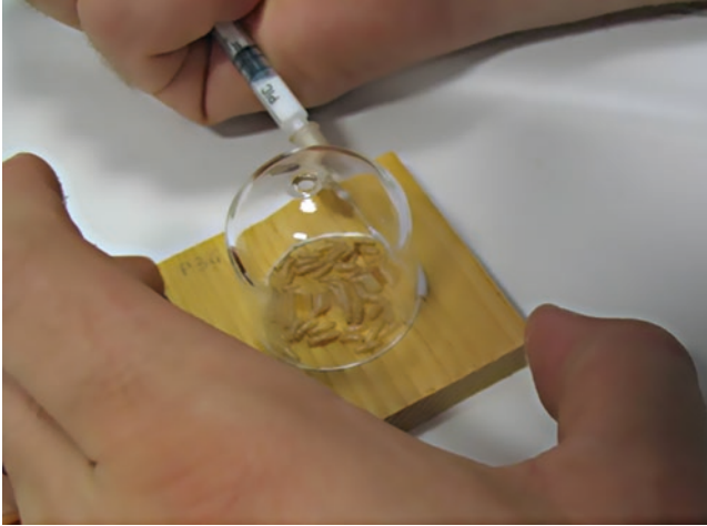
Fig. 12.3 Usage of the glue to secure with an adhesive the ground glass end of dome to the centre of the surface of the test specimen
