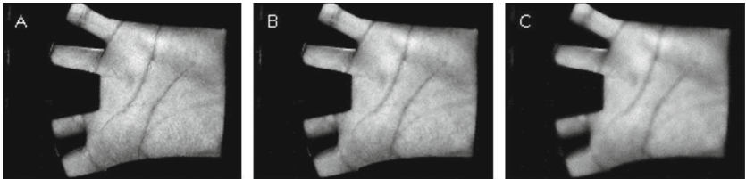
Fig. 3. Bilateral filter results with changing parameters \sigma_s and \sigma_r : A: \sigma_s = 5 and \sigma_r = 5 , B: \sigma_s = 25 and \sigma_r = 25 , C: \sigma_s = 75 and \sigma_r = 75
