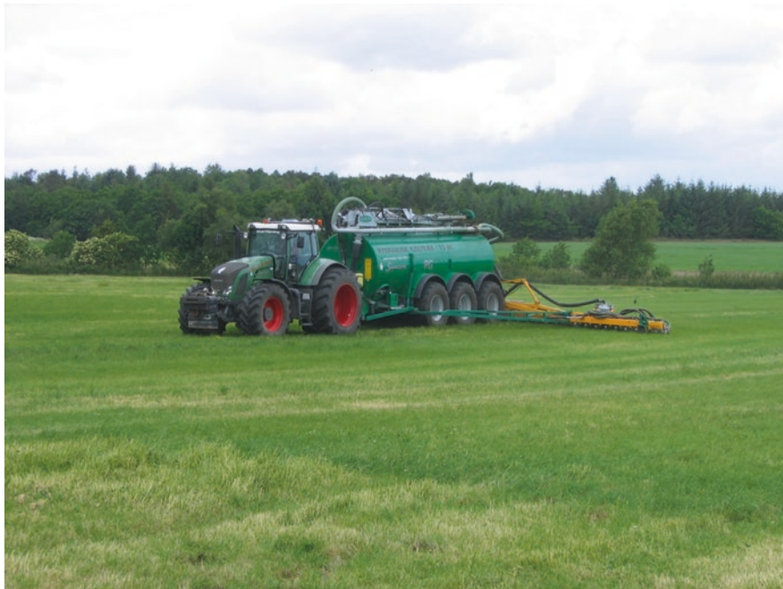
Fig. 7.4 Slurry tanker (14.5 m width) using a trailing shoe in CTF
