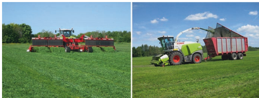
Fig. 7.3 A CTF system for grass silage (12-m width) at Moosegården in Denmark
