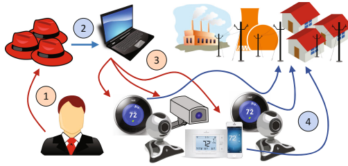
Fig. 1. Conceptual diagram of a PDoS attack. (1) Attack sponsor hires botnet herder. (2) Botnet herder uses server to manage recruitment. (3) Malware scans for vulnerable IoT devices and begins cascading infection. (4) Botnet herder uses devices ( e.g. , HVAC controllers) to deplete bandwidth of a cyber-physical service ( e.g. , electrical power).
