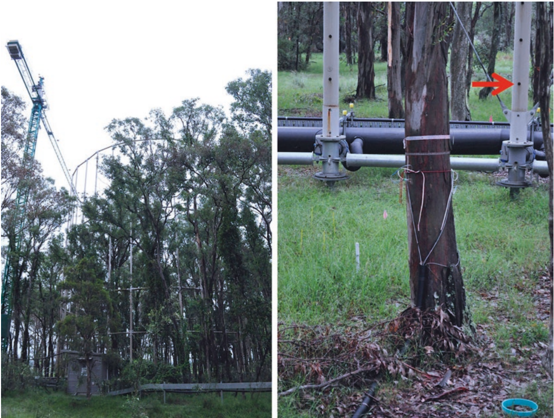
Fig. 4.3. Example of Free Air Carbon Dioxide (CO 2 ) Enrichment (FACE) technology at the EucFACE. (Left) Photograph of a CO 2 enrichment ring at the EucFACE experiment in Richmond, NSW, Australia. The ring encompasses an entire section a Eucalyptus forest. Pipes deliver CO 2 to each ring, where it is distributed throughout the center of the ring to achieve 550 ppm CO 2 . The photograph also shows a canopy access crane used for taking upper canopy samples (photo credit: Jeff Dukes). (Right) Close up view of the pipes that deliver CO 2 throughout the ring. A red arrow marks a hole from which CO 2 is released. A dendrometer band for measuring tree growth and a soil respiration collar are also pictured (photo credit: Jeff Dukes)
