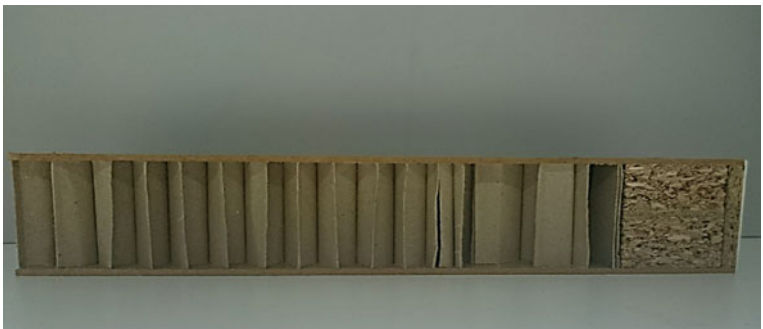
Fig. 15 Sandwich panel with paper honeycomb core
