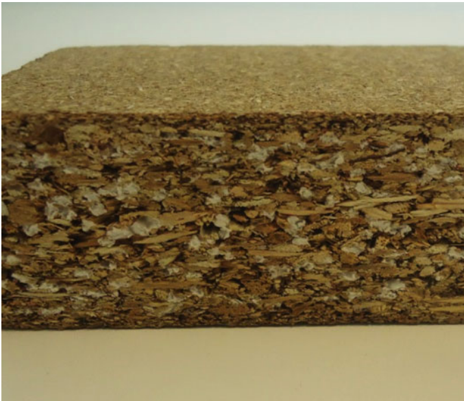
Fig. 8 Internal section of particleboard produced with expanded polystyrene foam (EPS) mixed with wood particles in core layer
