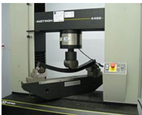
Fig. 26 Flexural test (Regional centre of animation in advanced materials 2004)
