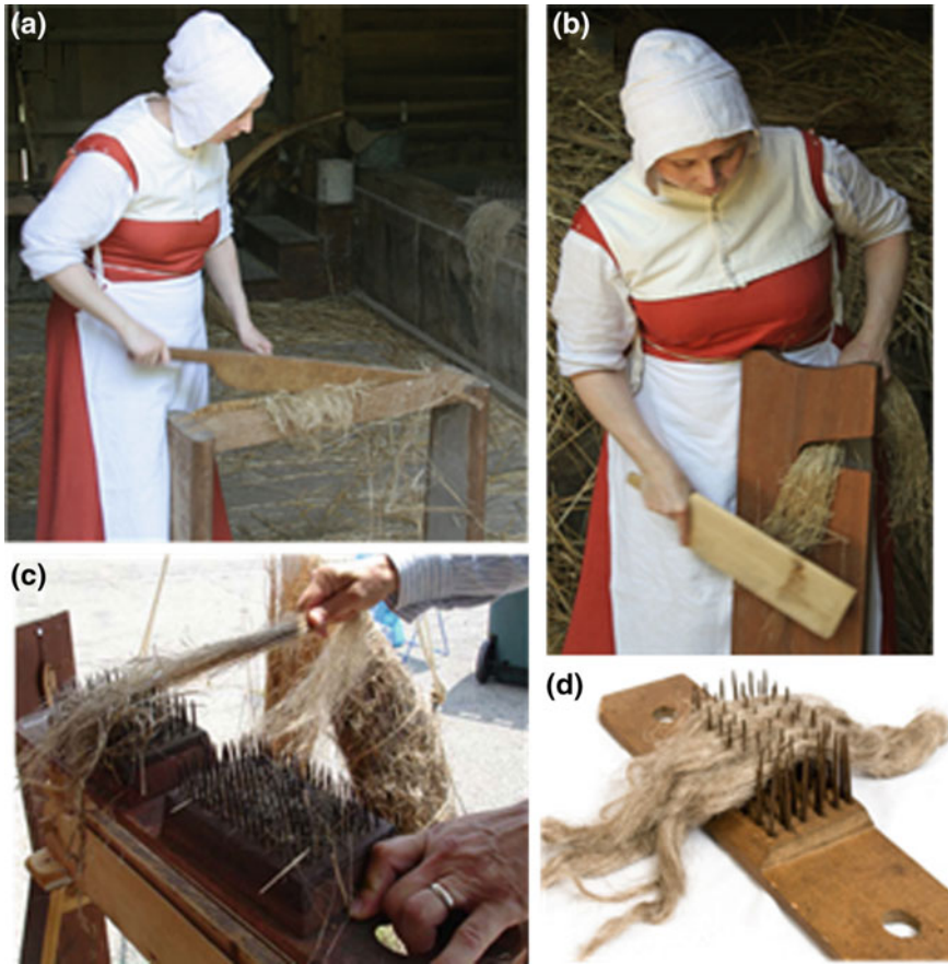
Fig. 6 Traditional retting of hemp fibers: scutching (a and b frames) and hackling (c and d frames) (Weald and Downland Open Air Museum 2016)
