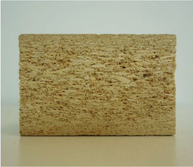
Fig. 7 Internal section of particleboard made from Populus spp. wood
