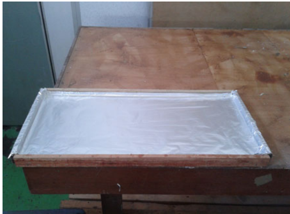
Fig. 17 Mould prepared for composite laptop table
