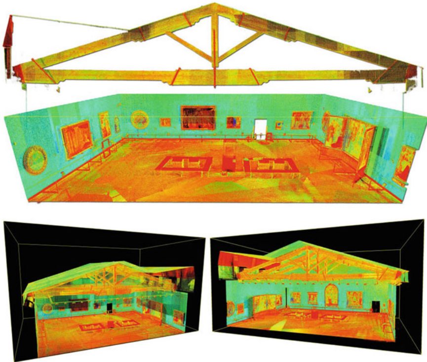
Fig. 9 Surveys carried out in the Botticelli room for the insertion of the new suspended ceiling
