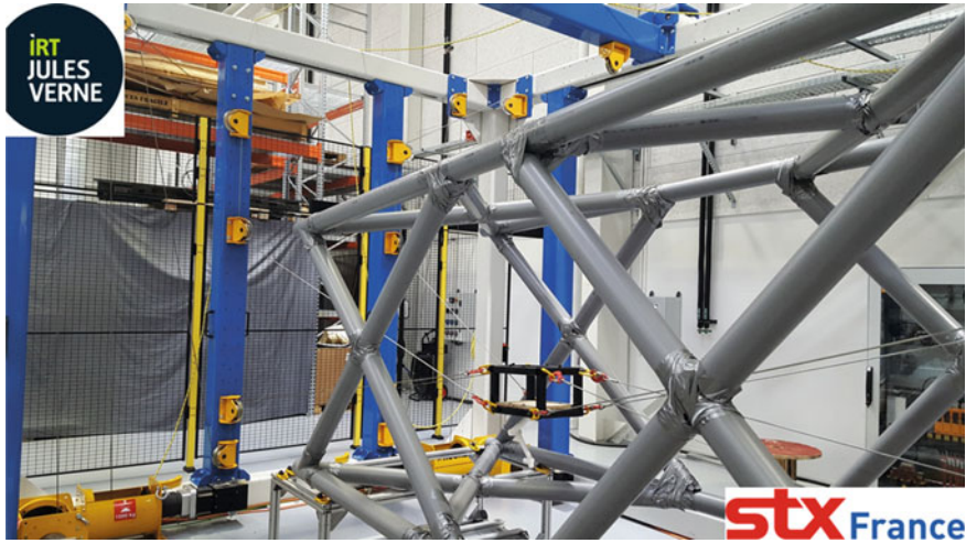
Fig. 2 CAROCA prototype: a reconfigurable cable-driven parallel robot working in a cluttered environment (Courtesy of IRT Jules Verne and STX France)
