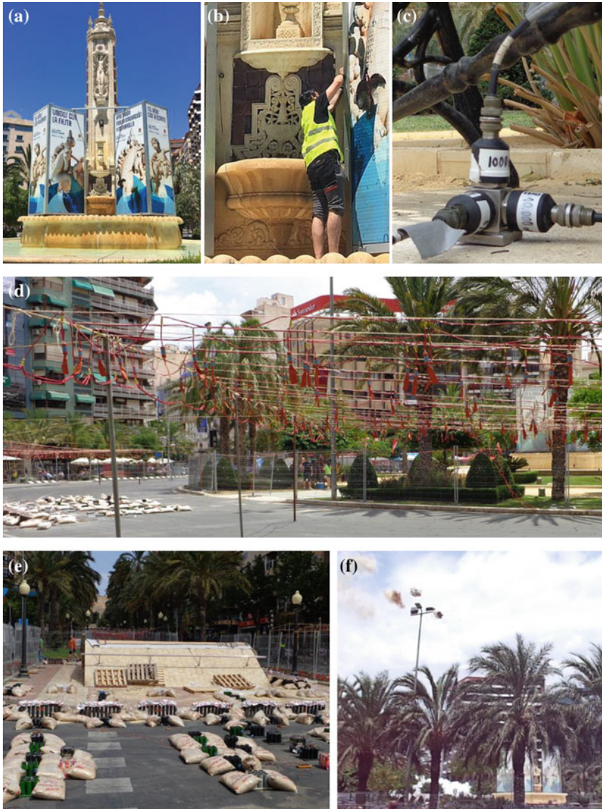
Fig. 6 a General view of the fountain and the protective screens; b sensor installation; c triaxial setup; d relative position of the fountain and explosives; e detail of the fireworks devices; f view of the fountain during the spectacle
