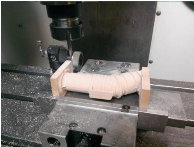
Fig. 7 Final machining stage of the connector on the milling machine
