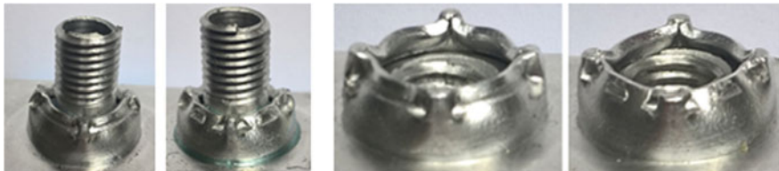
Fig. 10 Photographs of the samples after the execution of the joint and after the strength test
