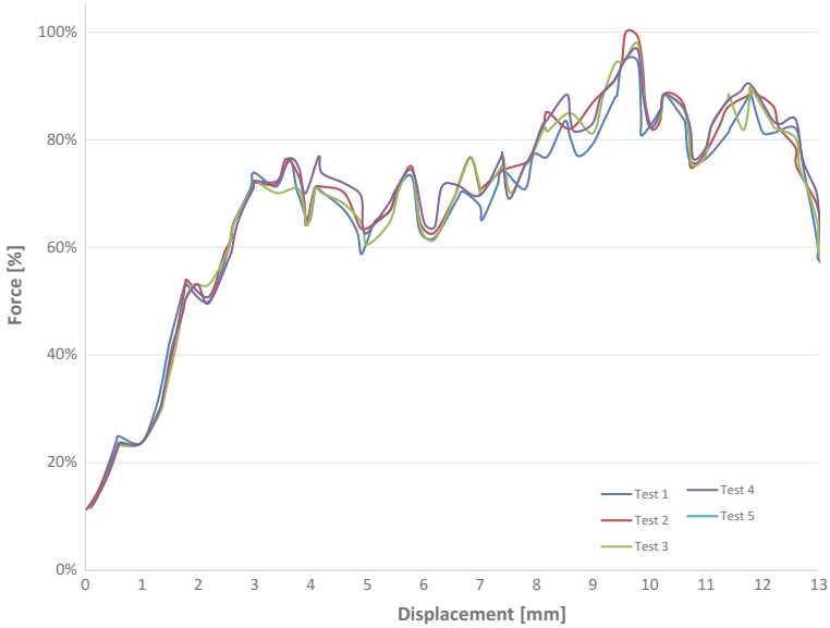
Fig. 4 Punch profile for F1 optimized geometry
