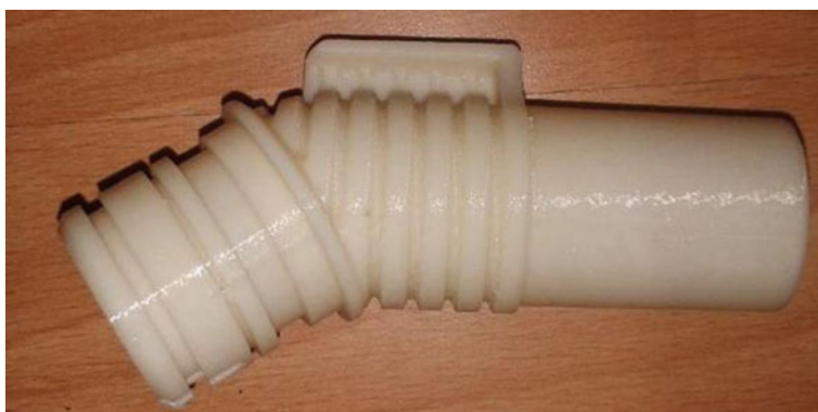
Fig. 5 Model of the connector performed on a 3D printer
