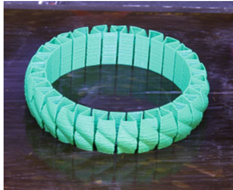
Fig. 2 Test print model—ABS bracelet
