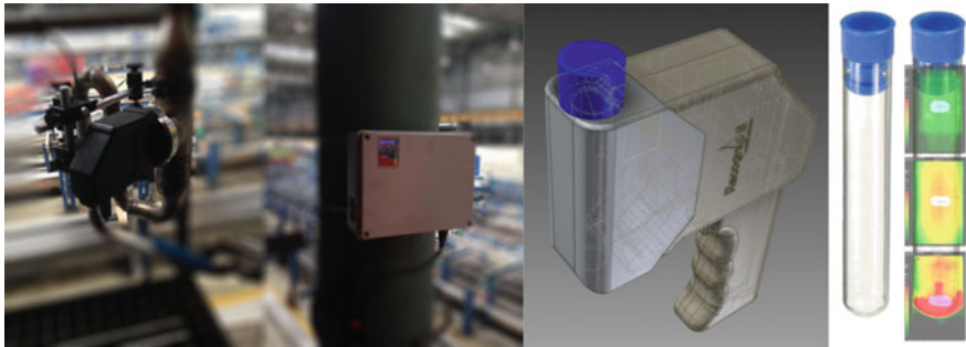
Fig. 9 Fluorescence measuring in bypass manufacturing (left), model of cover for field measurements of collected fluid samples (center), measurement outputs (right)
