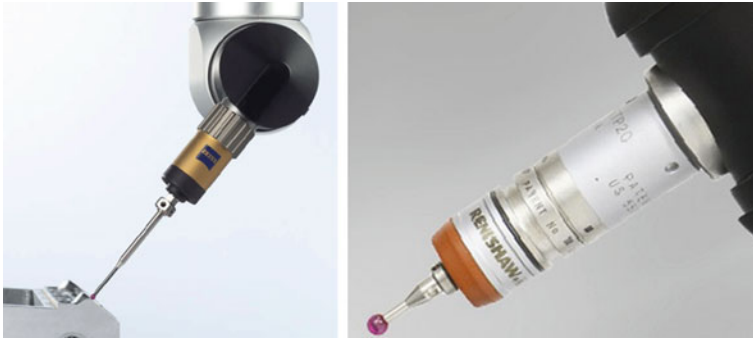
Fig. 2 Left picture presents RST-P [7], right picture presents TP20 [8]
