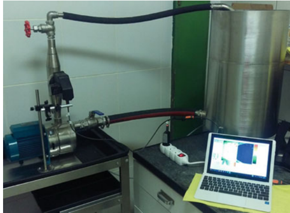
Fig. 8 Laboratory loop for measurement of contamination of working fluids (EVERSTAR, s.r.o.)
