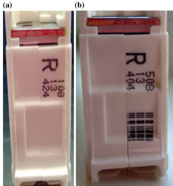
Fig. 2 Example of chambers: a correct (without gap) and b defective (with gap)
