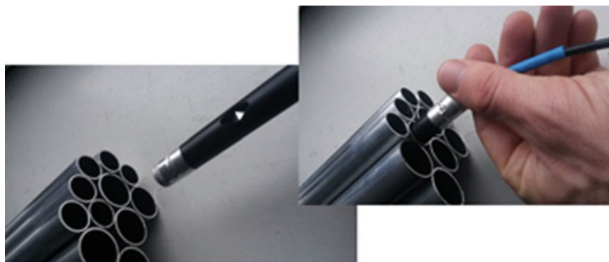
Fig. 5 Measuring of greasy contamination of inner tube surfaces
