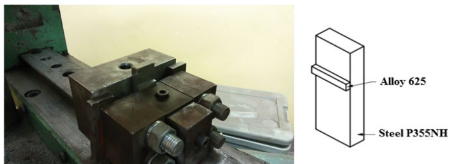
Fig. 2 Specimen with technological set prepared for shear test
