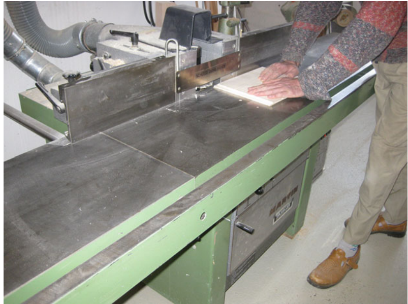
Fig. 1 Extraction machinery minimizing exposure to wood dust
